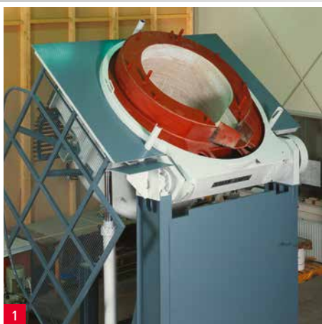
Basic design Vacuum tight, tiltable, charge weights up to 30 tons
