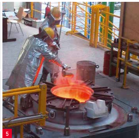
Pouring VID-Pro Pouring under protective gas [4]
