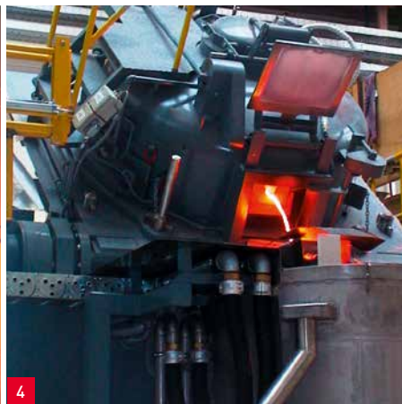
Pouring VID-Pro Pouring under protective gas [4]
